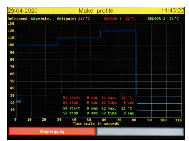
3. Once the **Stop logging** button is replaced by two other buttons, **Clear screen** and **Save log data**, you can remove the product from the belt and disconnect the sensor(s).
